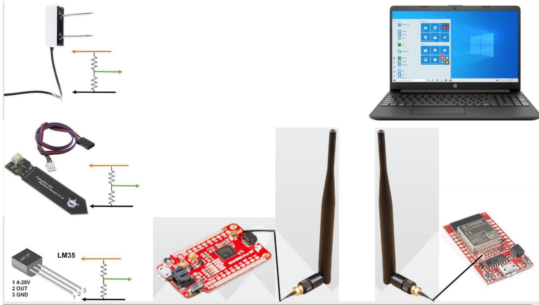
Figure K.1. Laboratory demonstration arrangement with transmitter, gateway, antennas, and host computer.
