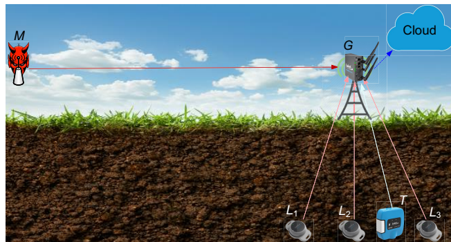
Fig. 1. Several underground nodes L securely bootstrap with the gateway G assisted by the trusted node T in the presence of an adversary M .
